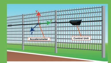
Accelerometer-based fence-mounted intrusion detection technology detects movement on fencing or walls based on an x, y, z axis system. Accelerometers sense dynamic forces of acceleration of the three axes combined, then measures detection signal intensity to trigger alarms.
