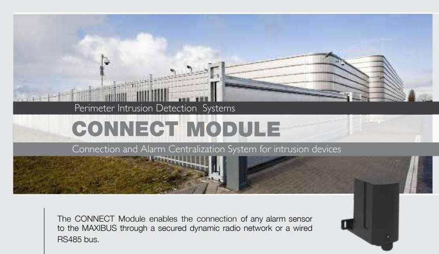
The CONNECT module is compliant with all dry contact outputs. MAXIBUS Universal becomes the unique interface to manage all alarm devices on site.
