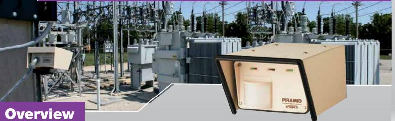
The PIRAMID XL2 outdoor intrusion sensor combines Stereo Doppler Microwave and Passive Infrared technologies whereby both technologies must activate simultaneously to create an alarm. The Stereo Doppler Microwave portion activates upon the movement of an intruder and the Passive Infrared portion activates on the change in infrared radiation caused by the intruder.
