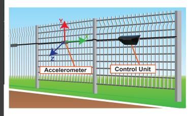
Accelerometer-based fence-mounted intrusion detection technology detects movement on fencing or walls based on an x, y, z axis system. Accelerometers sense dynamic forces of acceleration of the three axes combined, then measures detection signal intensity to trigger alarms.
